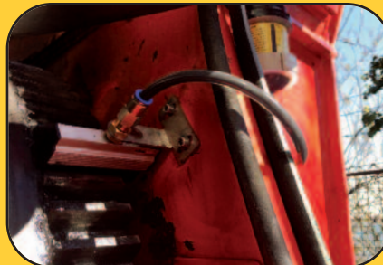
Open Gears – Brush application
